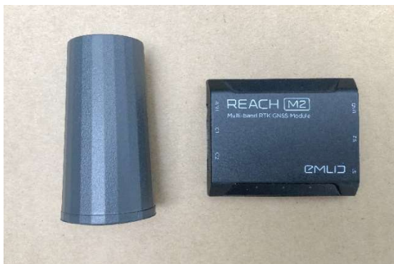
Image: Emlid Reach M2 Module and Antenna. Not included in the kit.
