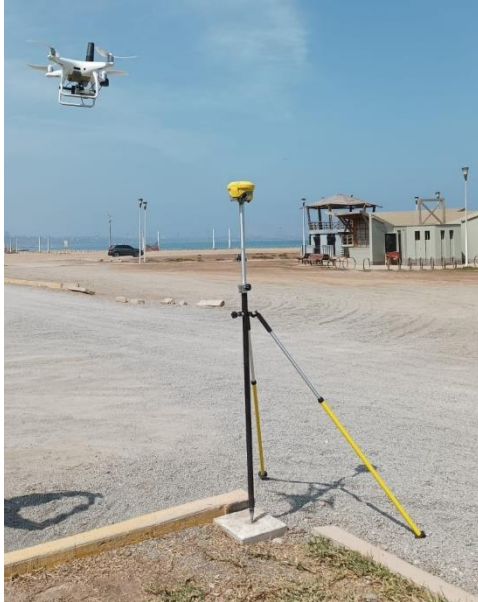
Figure 03: Geomax Zenith 35 and Phantom 4 base receiver with X5 Multiband GNSS Module.
