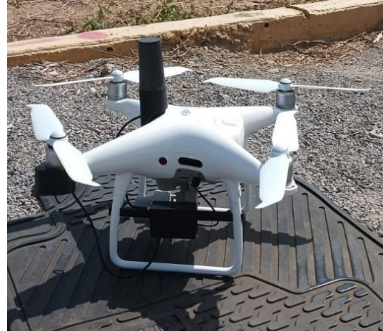
Figure 03: Geomax Zenith 35 and Phantom 4 base receiver with X5 Multiband GNSS Module.
